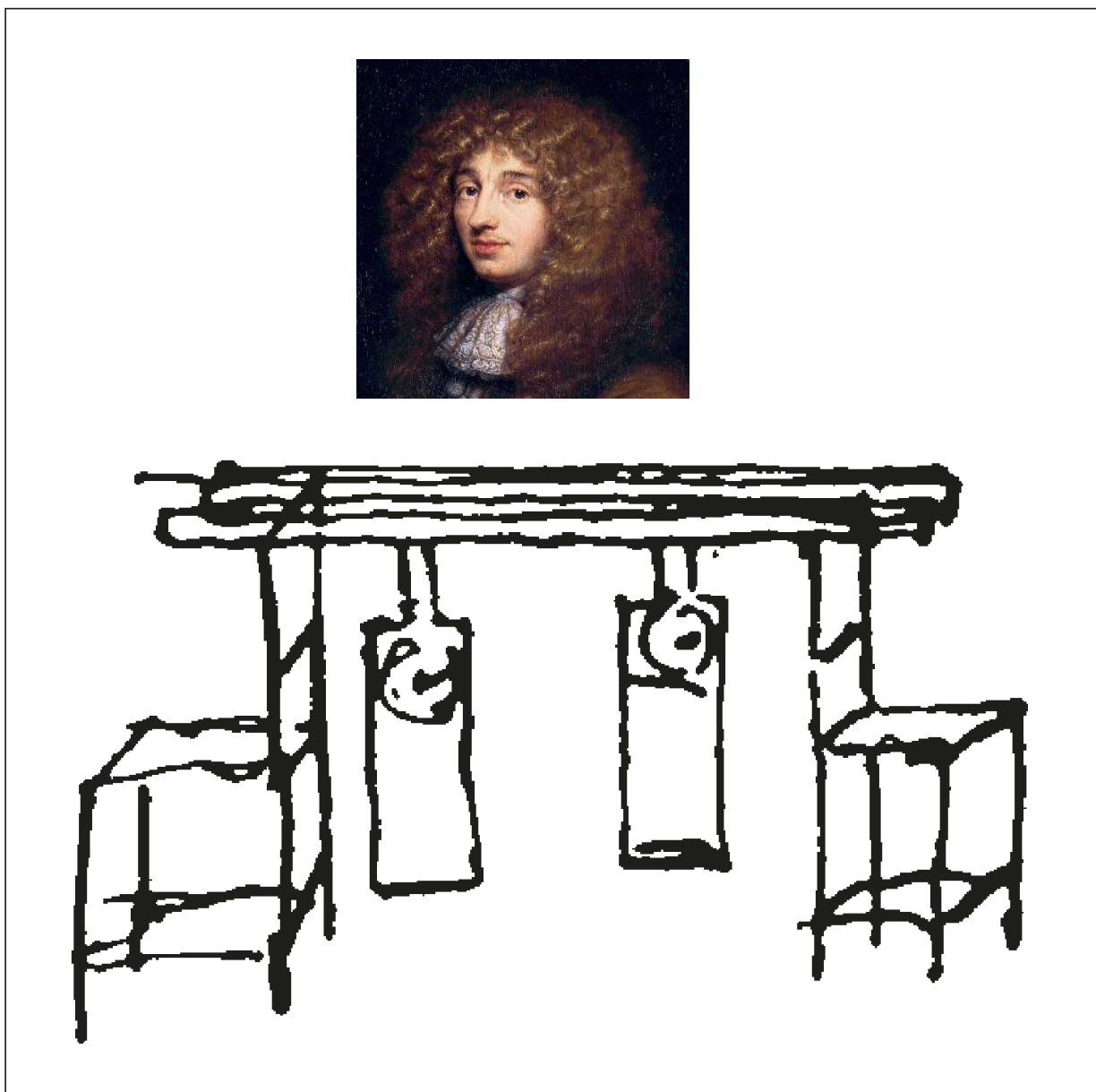
Fig. 1 Christiaan HUYGENS (1671) and his sketch of the two coupled pendulum clocks which he observed to synchronize spontaneously. (After HUYGENS 1932.)
