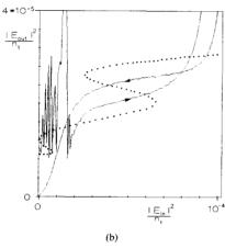
Fig. 4. Optical bistability: normalized optical output intensity is plotted versus optical input intensity for  $J=1.2~J_r(J_r$  threshold current density),  $\omega_{\rm in}=0.25,~\alpha=7$ , and (a)  $t_C=33$  ns and (b)  $t_C=4$  ns. (Full line: time-dependent numerical solution, dotted line: static analytical solution.)
