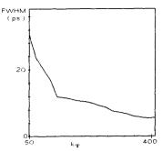
Fig. 12. Dynamics of pulse-compression: FWHM of output intensity is plotted versus index  $k_T$  that labels subsequent pulses, corresponding to number of round trips in ring configuration ( $\alpha = 0$ ,  $R_{\rm ext} = 0.5$ ,  $J_{\rm max} = 0.54$ ,  $J_{\rm t} = 2.8$ ,  $J_{0.33}$ ,  $R_{1.2} = 10^{-5}$ ).
