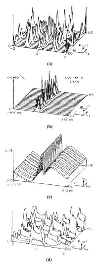
Fig. 7. Simulation for periodic injection current without feedback.  $(J_{max} = 6.1 J_I, \alpha = 0, \omega' = (\omega - \omega_0)/\Delta \omega_{\rm FP}$  is normalized frequency,  $k_T \in \mathbb{N}$  is index that labels subsequent emitted pulses, t' is time scale for one pulse with total elapsed time  $t = k_T T_J + t'$ , and  $-T_J/2 < t' \le T_J/2$ .) (a) Power spectrum of output field
