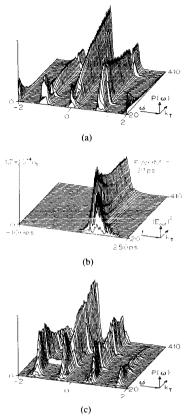
Fig. 10. Simulation of ring configuration with low feedback and low reflectivities (same parameters as in Fig. 9, but with  $R_{1,2} = 0.01$ ,  $J_{\text{max}} = 1.35 J_t = 2.8 J_{0.33}$ , where  $J_{0.33}$  is the injection current threshold for reflectivities of 0.33). (a) Power spectrum. (b) Temporal evolution of the output intensity. (c) Influence of the linewidth enhancement factor in mode-locking regime (same plot as in (a), but with  $\alpha = 3$  instead of  $\alpha = 0$ ).
