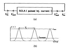
Fig. 6. (a) Scheme of ring configuration. (b) Injection current versus time.
