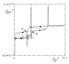
Fig. 5. Optical tristability, plotted as in Fig. 4, with  $J=4J_t$ ,  $\omega_{\rm in}'=-0.5$ ,  $\alpha=7$ ,  $t_C=16$  ns, and maximum  $|E_{\rm in}|^2=10^{-3} n_t$ .
