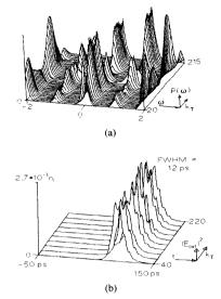
Fig. 8. Simulation of ring configuration with low feedback and high reflectivities (same parameters as in Fig. 7(a)–(c), but  $R_{\rm ext}=0.1$  and lower maximum injection current ( $J_{\rm max}=4.5\,J_{\rm r}$ ) in accordance with decreased effective dynamic threshold). (a) Power spectrum of output field. (b) Temporal evolution of output intensity.
