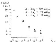
Fig. 11. Pulsewidth versus reflectivities for different gain linewidths  $\Delta \omega_g$  ( $\alpha=0$ ,  $R_{\rm ext}=0.5$ ,  $J_{\rm max}=0.54~J_t=2.8~J_{0.33}$ ).
