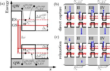
**Fig. 5:** (a) Energy diagram of the QD-QW system. (b) and (c) show direct electron capture and relaxation processes, respectively, from the QW to the GS (I,II) and the ES (III,IV). Panels I, III and panels II, IV show pure e-e and mixed e-h scattering processes, respectively. After [P3].
