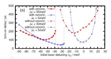
**Fig. 3**: Turn-on delay vs. initial cavity detuning with (solid) and without (dashed) many-body effects for inhomogeneous broadening of 5 and 30 meV. After [P1].
