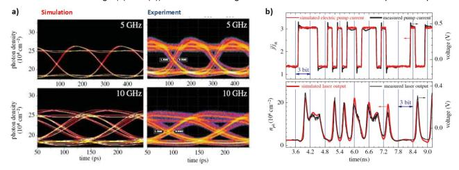
**Fig. 1:** (a) Simulated and measured eye pattern diagrams for pump currents switching between 4  $j_{th}$  and 6  $j_{th}$  ( $j_{th}$ : threshold current density) for bit repetition frequencies of 5 GHz and 10 GHz (b) Simulated (red line) and measured (black line) laser output (bottom) driven by an electric pump signal (top). After [P2].
