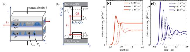
**Fig. 2:** (a) Sketch of the QD laser structure and (b) of the resulting energy band diagram. (c) and (d) show time series of the photon density during laser turn-on for different n-doping density (c) and different p-doping density (d). Dotted, dashed and solid lines correspond to doping of 0.1, 0.2 and 0.4 times the degeneracy concentration, respectively. Pump current  $j = 2.5 j_{th}$ . After [P2, P5].
