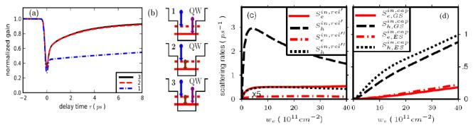
**Fig. 6:** (a) Ultrafast gain dynamics of QD optical amplifier for scattering scenario 1 (dash-dotted), 2 (dashed) and 3 (solid) as sketched in (b). Panels (c) and (d): Microscopically calculated Coulomb relaxation in-scattering processes between ES and GS  $S_{e/h}^{in,rel}$ , and in-scattering rates for capture into GS and ES  $S_{e/h,GS/ES}^{in,cap}$ , respectively, vs. QW carrier densities. After [P3].
