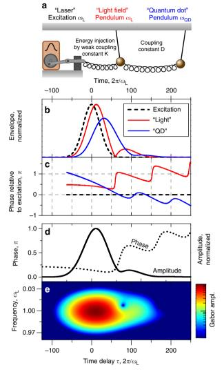
Figure 3 | Mechanical coupled oscillator analogue. (a) A qualitative analogue of the coupled light field-QD dynamics by two coupled pendula. (b,c) Amplitude and phase of the driving excitation (black), the light pendulum (red) and the QD pendulum (blue). (d) Envelope and relative phase of the convolution of excitation dynamics and light pendulum dynamics. The fast oscillations are removed. (e) Gabor surface derived for the data of d.
