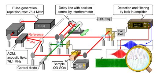
**Figure 1 | Experimental method.** Schematic of the FROSCH set-up for electric field cross-correlation measurement of fs pulses. To illustrate the time resolution of the method, the inset shows a zoom into a representative set of data, the real (blue) and imaginary (red) part of the lock-in signal and the interference pattern of the reference diode with a wavelength of  $\lambda = 780 \, \text{nm}$  (green).
