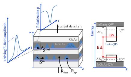
Figure 1. Schematic picture of the QD SOA and associated energy diagram (right) of the QD and QW systems.
